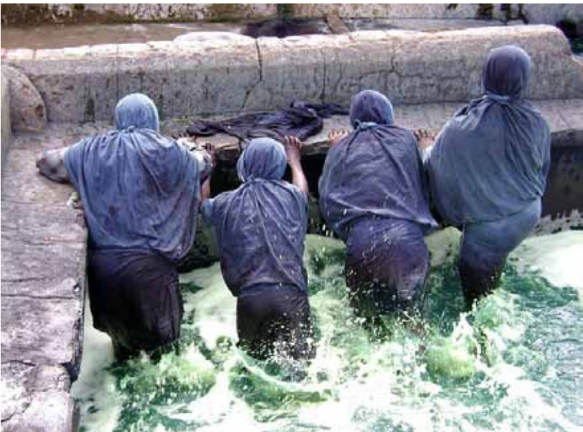
Workers kicking indigo liquid to oxidize it, Tamil Nadu, India. Foto: Mary Lance (bron: bluealchemyindigo.com)
